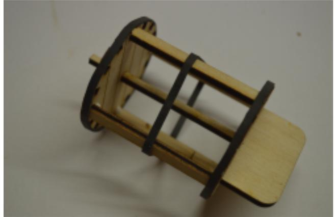
Assemble the rest of the slats onto the inner end pieces ensuring that the assembly is properly aligned and secure with an elastic band until the glue dries.
